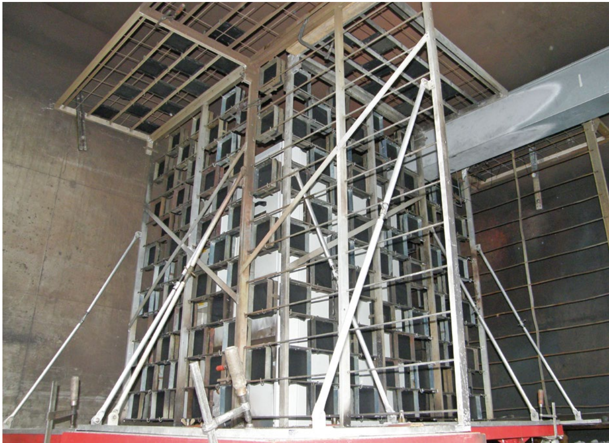
Setup for an internal arc withstand test
